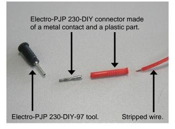
3 / 7. I introduce the wire into the plastic part, the trumpet side is opposite to the stripped end.
