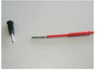
5 / 7. I introduce the metal contact into the 230-DIY-97 tool metal tube.
