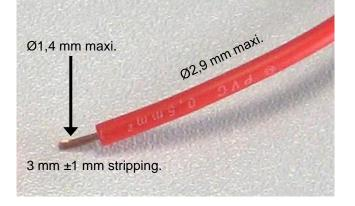
2/7. I strip the end of the wire by 3 mm typically (3 mm  $\pm 1$  mm) with the stripping tool.
